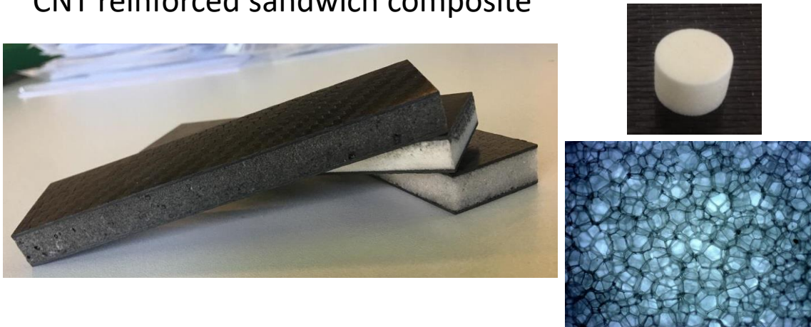
Functional Foams: Polymethacrylimide (PMI) foams/ CNT reinforced sandwich composite
